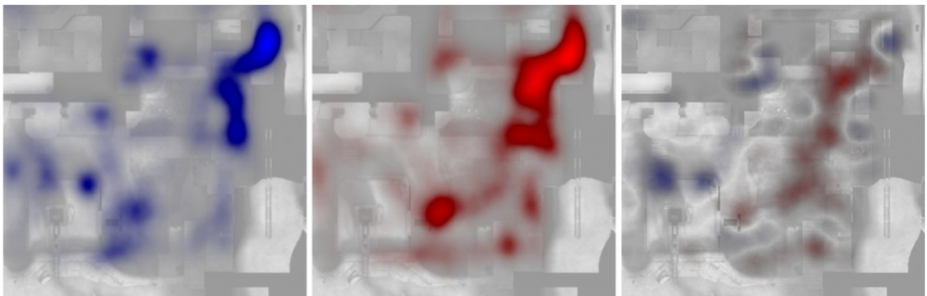
Figure 3. Two heatmaps can be combined into a single heatmap (right) by subtracting the values of one heatmap (middle) from the values of the other heatmap (left). (Based on Houghton, 2011)
